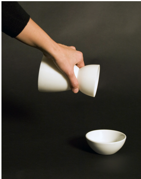
Figure 5.2: When a user tilts the Flops, a number of virtual items, that can only be heard, are poured out.
