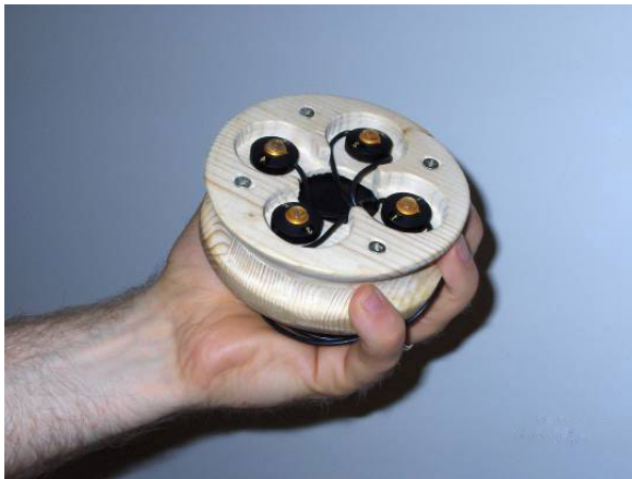
Figure 21.7: The hemispherical wooden device with fixed IR-Markers, used as a tangible device in the sports-related applications of AcouMotion.
